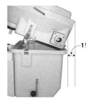
Be sure that the lid will open fully. You must also be certain that the bowl has enough room to tilt rearward to allow for its removal and for the removal of the 11/4" liquid tank.
