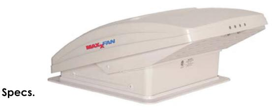
Fits 14"x14" roof opening Over 900 CFM Operation - Remote or Manual 10 Speed Intake and exhaust fan 12" blade fan Fuse protected 12v motor
