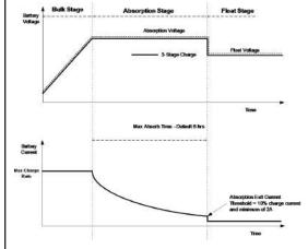
**NOTE**: When the charge cycle is interrupted, the charger will restart charging at the beginning of the multistage algorithm. Charge current during equalize state (optional state not shown here) is normally limited to 10A for 60 min.
