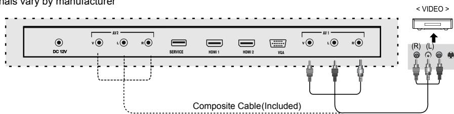
Connect the LED TV'S Composite In terminal to VCR's Composite OUT terminal using the included Composite cable.
