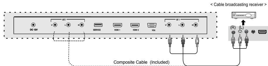
Connect the LED TV's Composite In terminal to the cable broadcasting receiver Composite Out terminal using the Composite cable. (Make sure the color of the terminals and the color of cable are the same)
