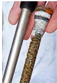
Figure 5 Good and Bad Anodes
